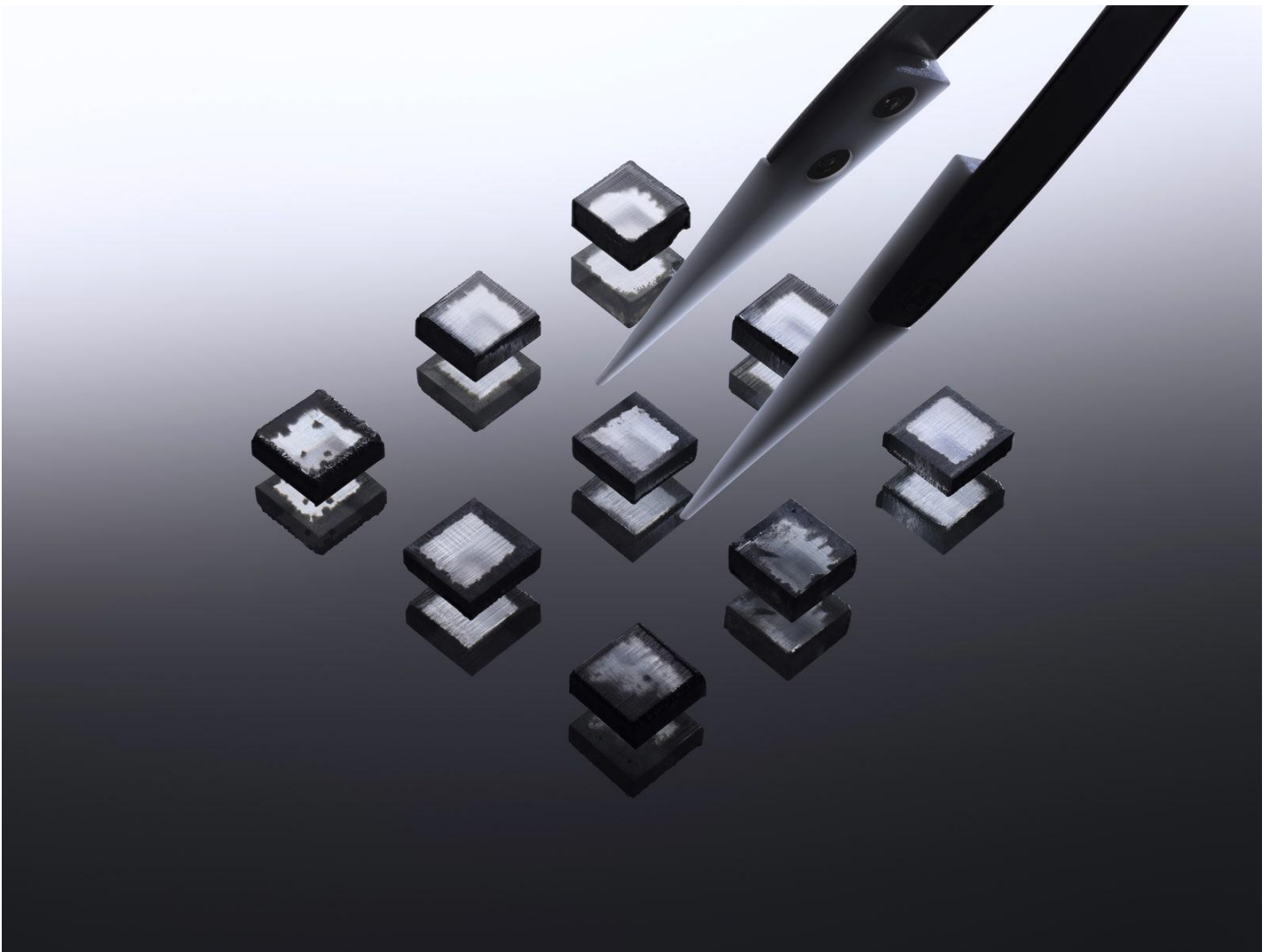
The raw unpolished lab-grown diamonds after they have been grown using chemical vapor deposition.
